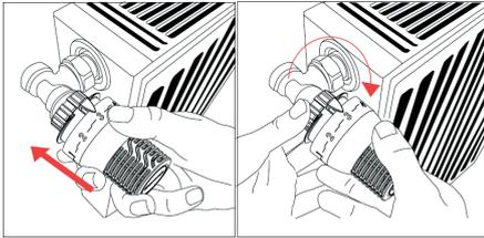
1. Place the index at position 5, in the vertical top position.
