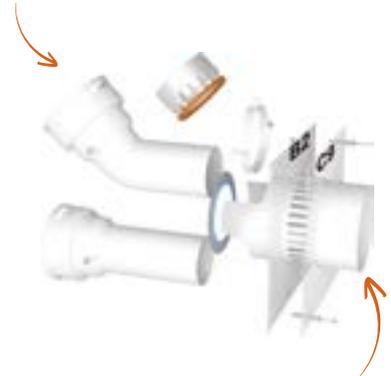
**Sortie Ø60/100 raccordement**
