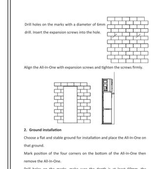
diameter of the holes is about 13-14 mm. The hole which closest to the
